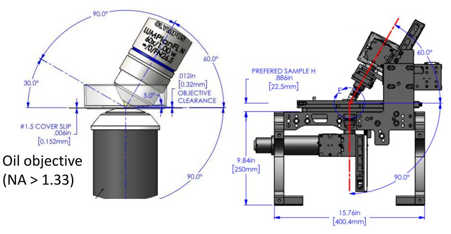
Bottom objective creates tilted light sheet for imaging with top objective
