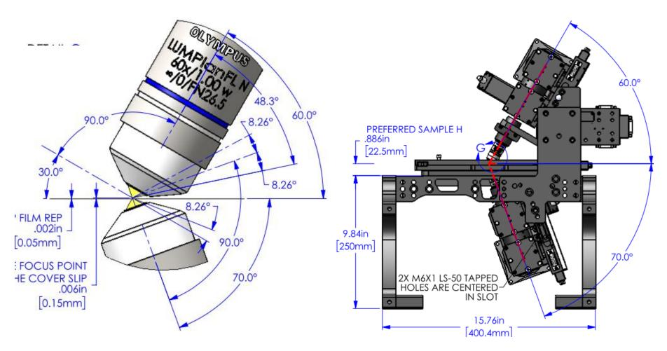
Dual-view system, objectives sequentially generate light sheet and image
